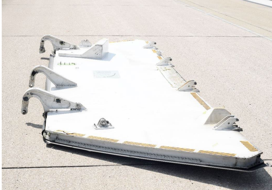
The Mishap Aircraft's LMLG door depicted on the runway following the mishap.
