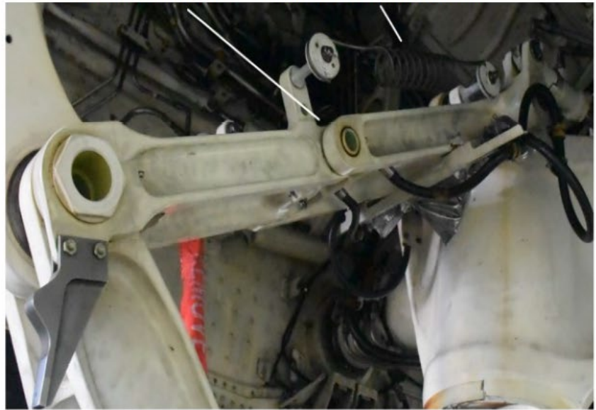
The function of a lock link illustrating the over center (locked) position.
