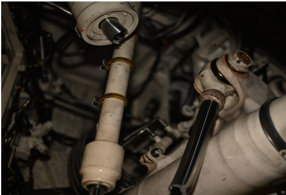
The LMLG's broken retract actuator piston depicted following the mishap.
